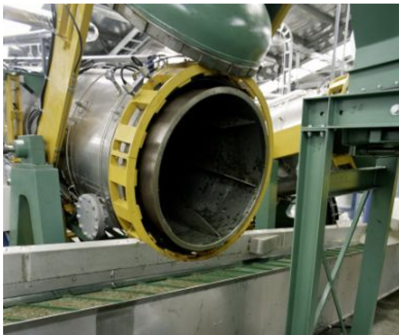
One of the mediclaves at Interwaste’s Seaview plant
